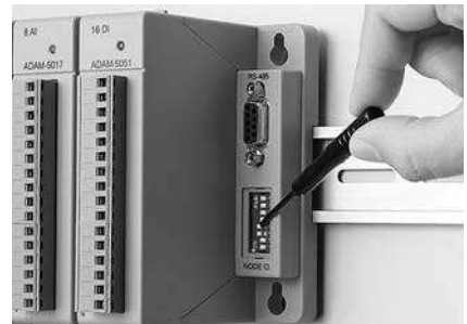
Node ID Setting 8-pin dip switch configuration
