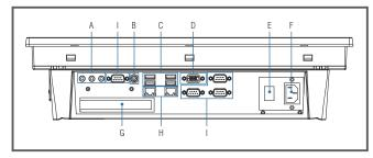
A: Line in/Line out/Mic in B: PS2 Mouse&Keyboard C: USB 2.0 x 4 D: VGA Port E: Power Switch F: AC Inlet G: PCI Slot x 1 H: 10/100/1000 Mbps Ethernet x 2 I: RS-232 x 3, RS-232/422/485 x 1
