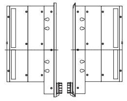
The flat-sealed front panel of IPPC-9151F-XAE (shown above left), is designed for minimum projection in panel mounts. This ensures easier liquid run-off, prevents dirty edges, and is useful in applications where hygiene is crucial (e.g. food processing).
