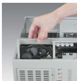
Easy-to-maintain cooling fan
