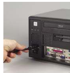
Plug ring-lock securely fastens the power cord
