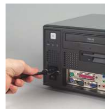
Plug ring-lock securely fastens the power cord
