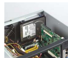
Shock-resistant drive bay for holding an internal 3.5" HDD
