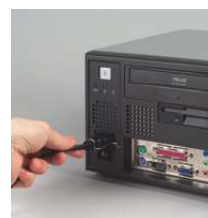
Plug ring-lock securely fastens the power cord
